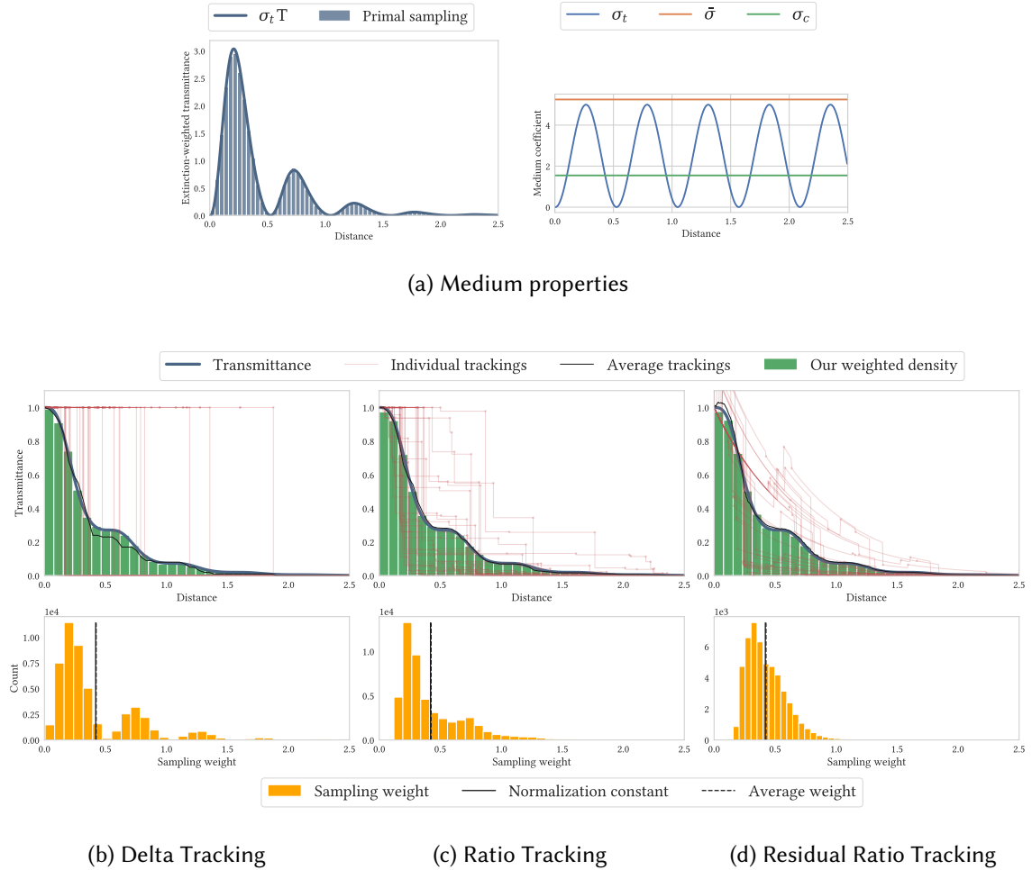
Figure 5.6: Demonstrating our novel transmittance sampling methods based on delta- and (residual) ratio tracking. (a, bottom) We use a 1D analytic medium with density following a sinusoidal function. The chosen majorant and control densities are also shown. (a, top) Forward rendering of such a medium involves sampling free-flight distances proportionally to \sigma_t(t) T(t) . Locations where \sigma_t \approx 0 receive few or no samples, which leads to bias and high variance when using this same sampling technique to estimate gradients. Instead, we propose dedicated transmittance sampling techniques for the adjoint. Delta tracking (b) , ratio tracking (c) and residual ratio tracking (d) can be interpreted as building estimates of the transmittance function using binary, piecewise constant and piecewise-exponential functions respectively. We build transmittance sampling algorithms from those trackers by sampling distances from their individual function approximations. They produce weighted samples (green histogram) with density equal to the transmittance function T , where the weights (yellow histogram) approximate the normalization constant of T .
